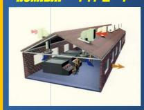
Units designed to work by overpressure. They are installed on the roof of the building and introduce the cooled air vertically. Each units incorporates its own motor-ventilator equipment.
