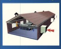
Units designed for large buildings via distribuiton tubes. Each unit is equipped with a motor-driven centrifugal ventilator. They can be installed either on the walls of the building or on the roof. The air is conducted and introduced via distribution tubes, driven by its centrifugal ventilator
