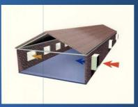
Units designed to work by overpressure. They are installed on the walls of the building, and introduce the cooled air horizontally. Each unit incorporates its own motor-ventilator equipment.
