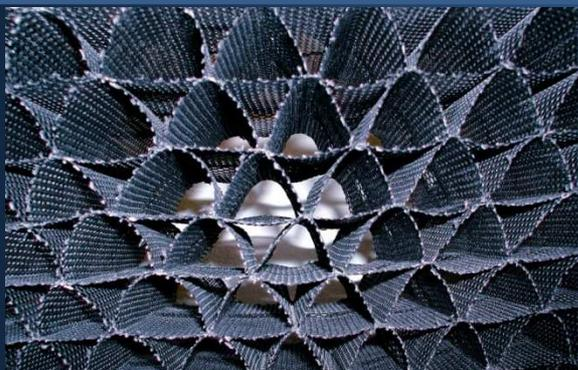
The comb is a support for a generate interface surface, so that starting with this basic concept finds it's field of activity in aplicaciones relacionadas with the transfer of heat and mass between liquid and air.
