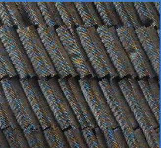
Otherwise, the canals, always straight, can be either parallel or oblique with respect to airflow. The first form are used on machines with vertical air circulation, as cooling towers, while the comb with oblique canals also called drift eliminator, is used for retention of drag liquid drops and for machines with horizontal air flow, as cooling evaporative, humidification sections of air treatment units, etc.
