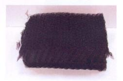
The average value for the water mass flow during the test was 5049.021/h and the air exit velocity average value was 3.77 m/s. A drift rate of 0.00623% of the circulating water flow is measured for Panal C & V Drift Eliminator. This value represents an emission level an order of magnitude lower than 0.05% which is the maximum value set by Spanish Law Real Decreto 865/2003, por el que se establecen los criterios higiénico-sanitarios para la prevención y control de la legionelosis.
